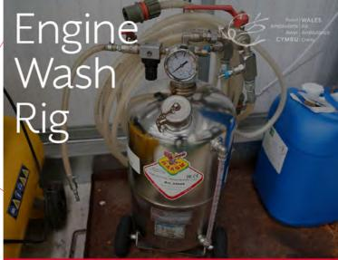
This engine wash rig allows us to send cleaning fluid into the engines, helping to prevent corrosion and dirt buildup.
